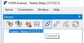
Now the client-server connection can be established: in **Server** window from context menu of the selected device invoke the command **Connect**
