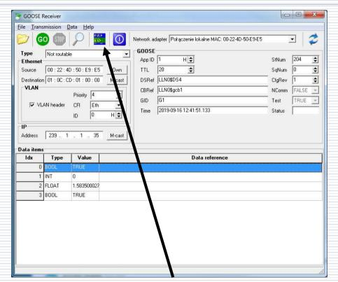
A sequence of received GOOSE messages can be traced in the invoked **Parser** window.
